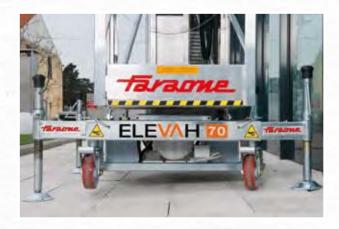
By using stabilizers and positioning the cage 70 cm above ground level, a working height of 7 m can be reached.
